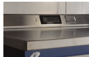
13: 3 power outlets (12A) for 15A circuit, 2 USB ports, a knockout for a pneumatic connection and a perforation (with cover plate) for installing a telephone or network jack
